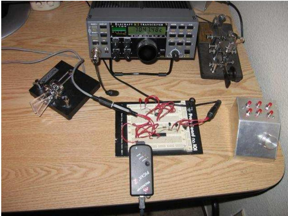
Figure 7: The prototyped PIC16F690-I/P circuit connected between the paddles and the K2. The CMOS Superkeyer III is the aluminum box with 6 pushbuttons to the right. The microprocessor is being powered by the PICkit 2 programmer shown connected to the in-circuit serial programming header.
